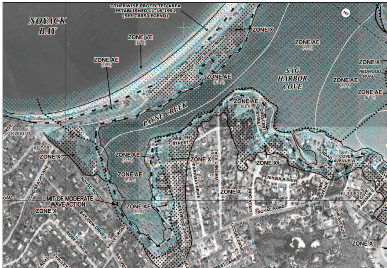
Figure 2-2. Typical DFIRM for coastal flooding showing the Limit of Moderate Wave Action (LimWA)
