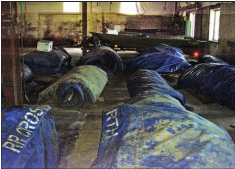
Figure 5D-40. Moveable floodwalls in storage that can be deployed by filling baffles with water
